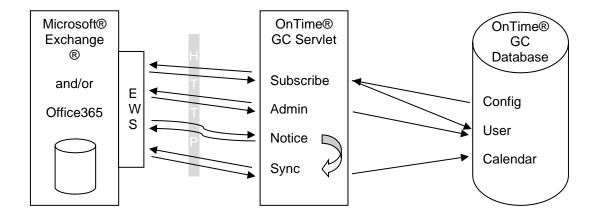
This illustration is to get an overview of the involved parts and shortly how they interact. It does not show the client-side, as this is identical to the HCL Domino® synchronisation, and data is stored in the same database.
