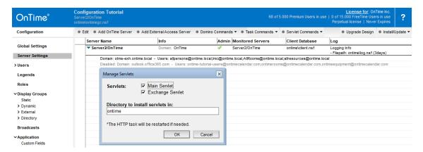
Add a check mark for 'Exchange Servlet' – do not remove the tick at the Main OnTime servlet, it will remove the already installed servlet. Clicking 'OK' do the following 4 steps:
